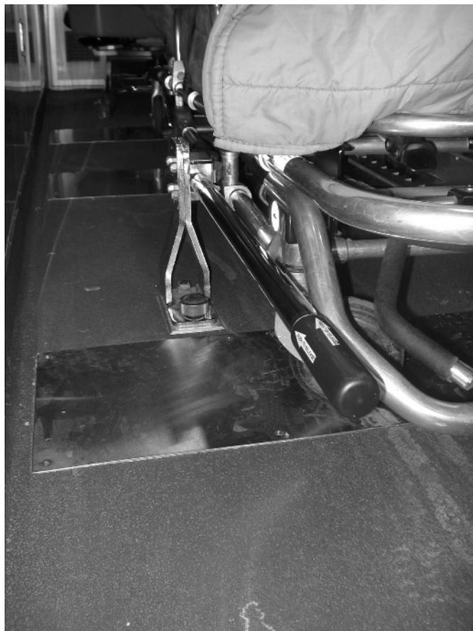
**Figure 3** Stretcher-fastening system. The mechanism secures the stretcher to the ambulance floor during transportation.
